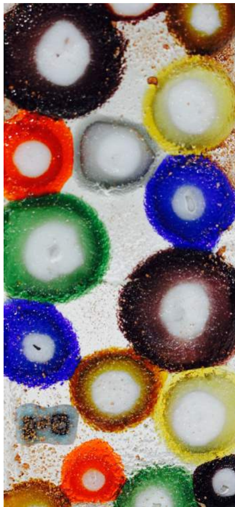
Figure 86 This test using surface transitional inclusions shows the visual difference between opaque white glass in the middle, opaque encased with a colour transparent glass on the next circle and on the outer rim of each circular inclusion the transparent only, 2014, photography credit J A Denton
