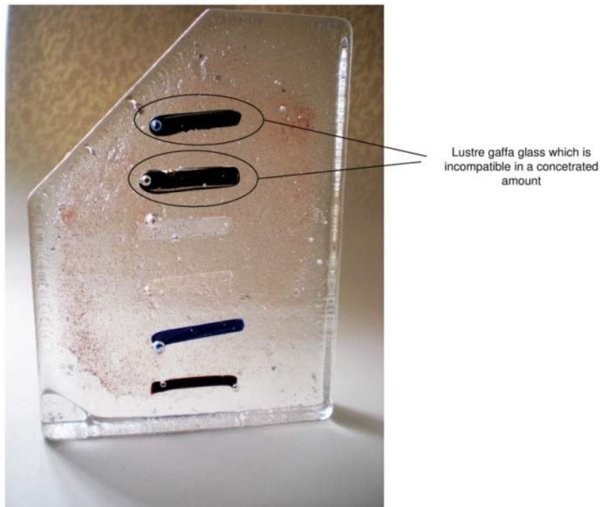
Figure 54 Gaffa lustre colour compatibility test, 2012, photography credit: J A Denton
