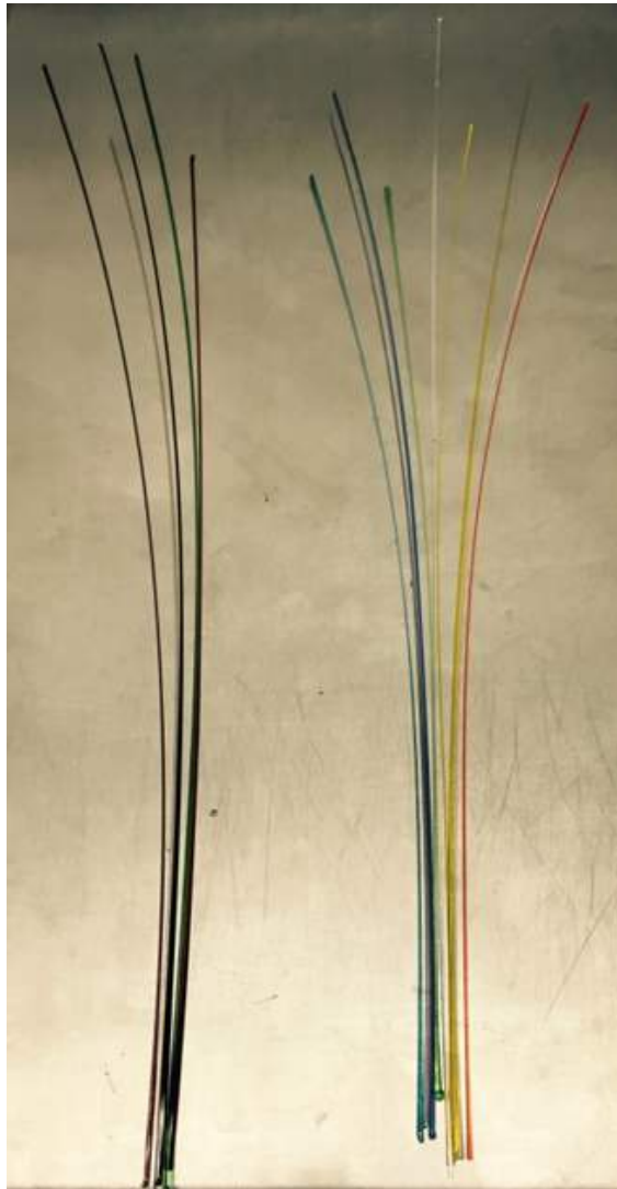
Figure 71 Compatibility pull test System 96 with clear Glasma furnace batch glass, 2015, photography credit: J A Denton
