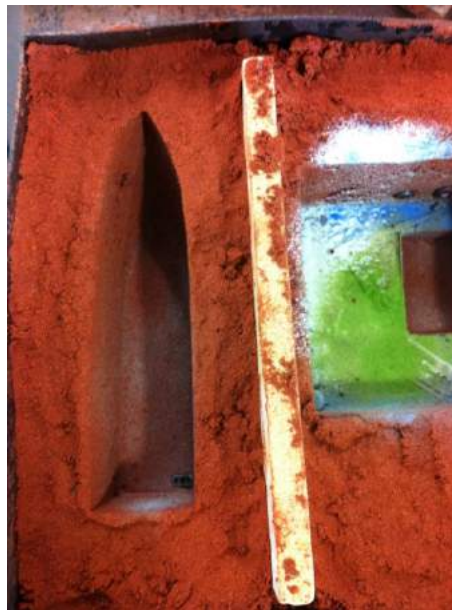
Figure 57 Negative forms separated by kiln shelf (or metal plate) pre-casting, 2014, photography credit: J A Denton
