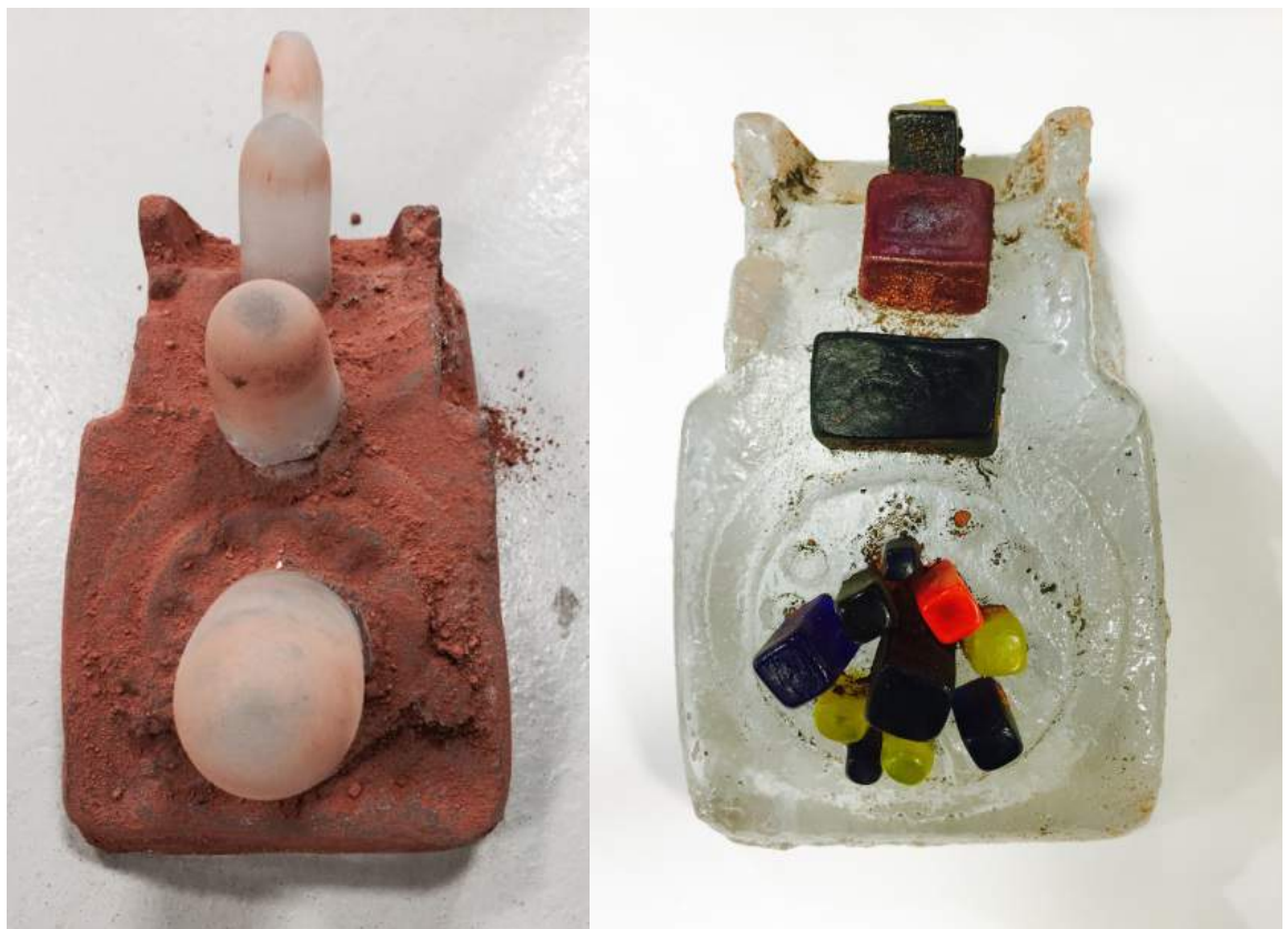
Figure 44 Visual difference between sandcasts made without a resist (left) and with a resist (right), 2015. Photography credit: J A Denton
