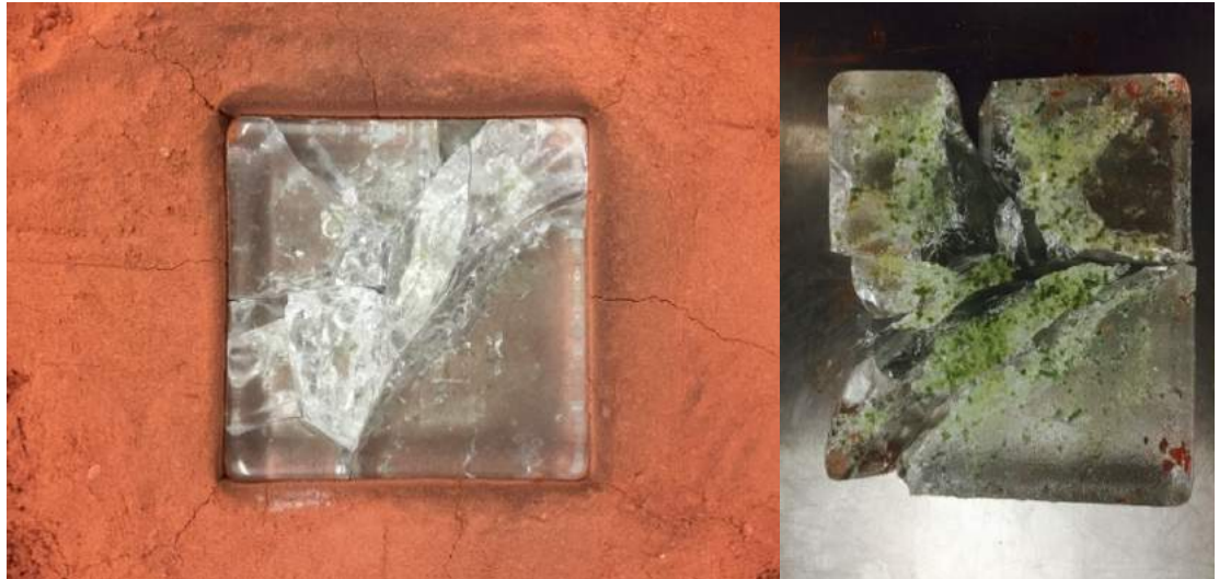
Figure 47 Incompatibility results when combining \alpha 32 borosilicate powder with \alpha 96 furnace glass, 2016, photography credit: J A Denton
