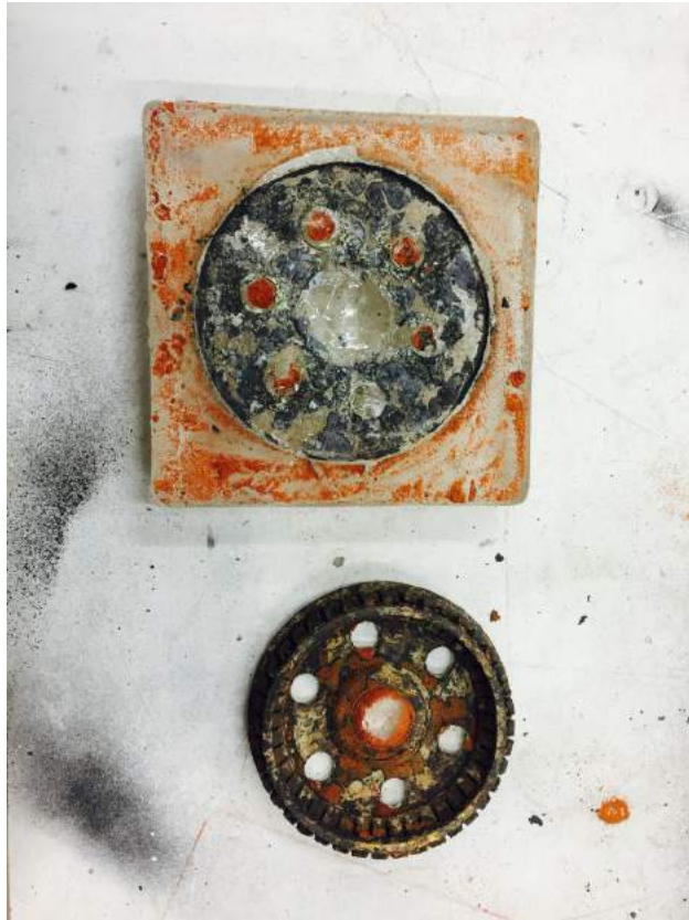
Figure 50 Large brass inclusion coated with ceramic release agent pre-casting and cast on the outside of the body of the sandcast like a transitional inclusion, 2016, photography credit: J A Denton
