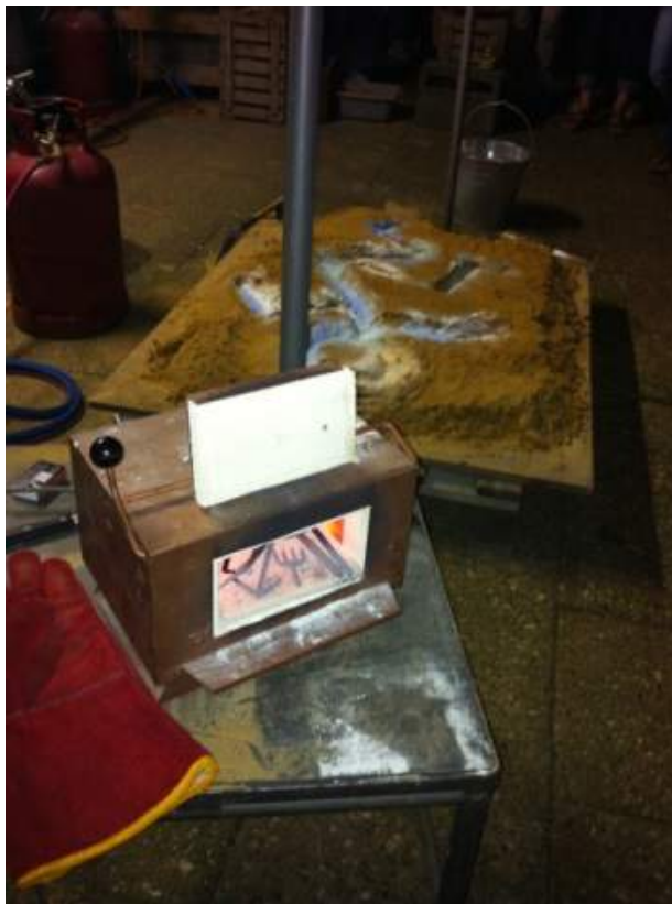
Figure 62 Flameworked inclusions painted with high fire enamels pre-heating before inclusion in freeform cast, 2015, photography credit: J A Denton
