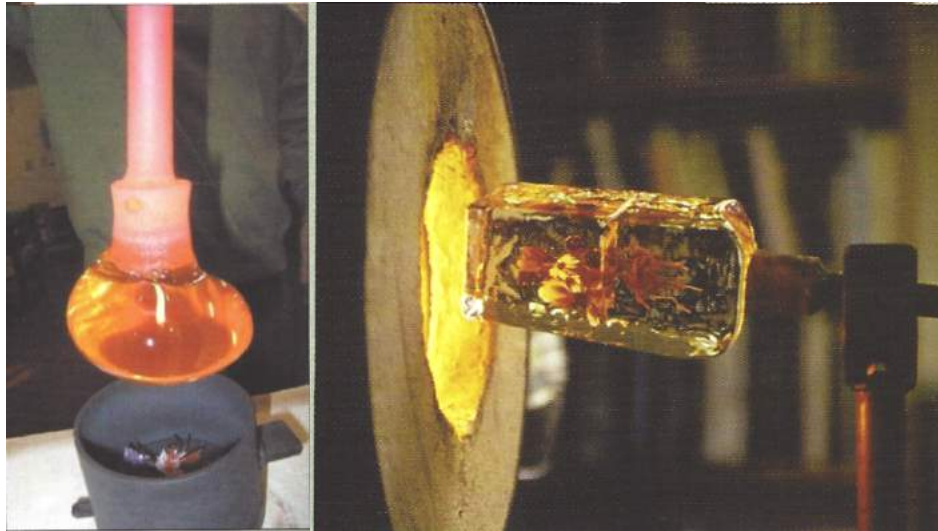
Figure 31 Left: Vacuum sealing components and right: Heating the finished paperweight, (Stankard & Eichhorn, 2007, p. Plate XVII & Plate XVIII), photography credit: Anon
