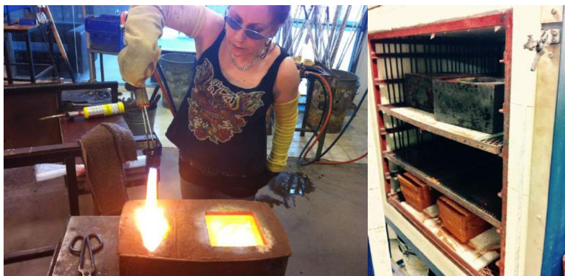
Figure 41 Example of two mould forms in a metal box almost ready to be placed in Lehr and after casting pieces annealing in the Lehr, 2012. Photography credit: Left: Anon. Right: J A Denton
