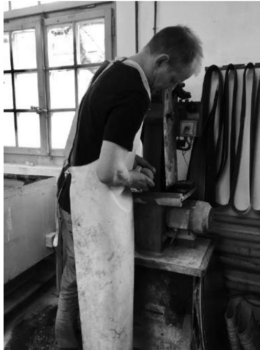
Figure 88 An example of one type of water-fed industrial polishing equipment being used by master glassblower Thomas Blank, 2017, photography credit: J A Denton
