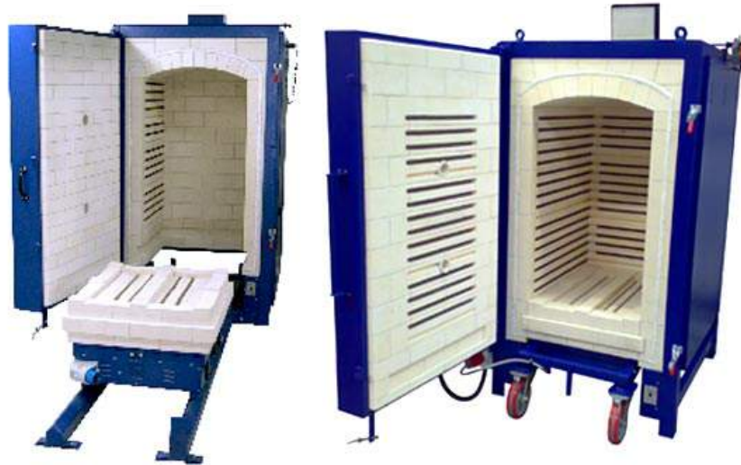
Figure 56 Example of a casting truck kiln with rollers, photography credit: Anon
