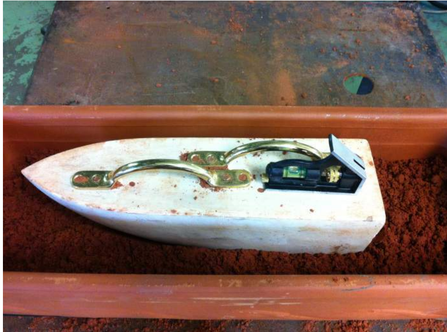
Figure 43 Example of plaster relief mould in the arch form placed on sand precasting.
