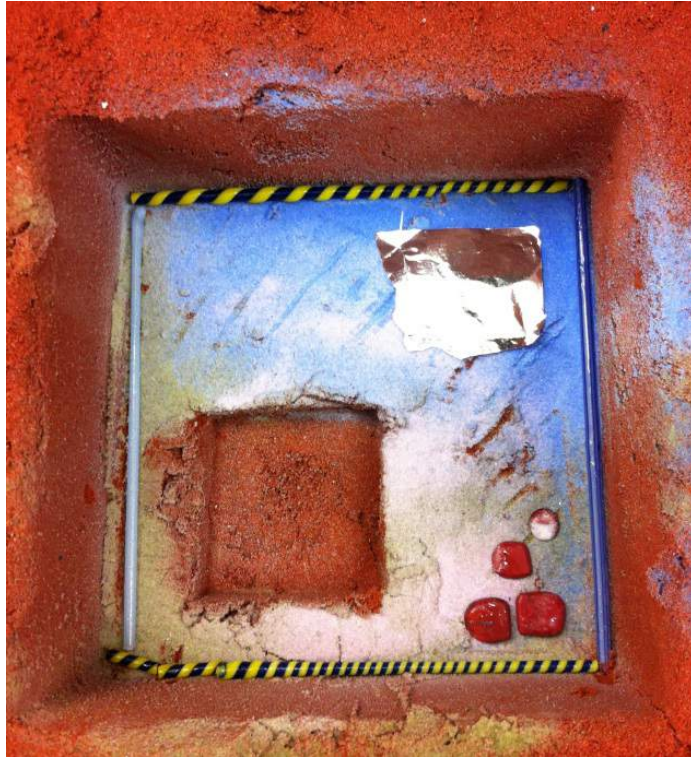
Figure 40 Example of use of powders and metal, plus use of cold inclusions on surface of cast leading to eventual discovery of the transitional inclusion technique, 2012.
