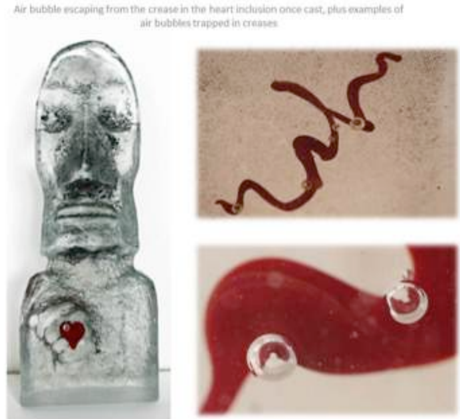
Figure 94 Example of unwanted air bubbles. Heartless Barstard series 'He's gotta lotta heart...' 2012 by J A Denton. Cast in sand mould with frameworked glass 'floating' inclusion; H. 45 cm, W. 24 cm, D. 7 cm, photography credit: Kevin Moonan
