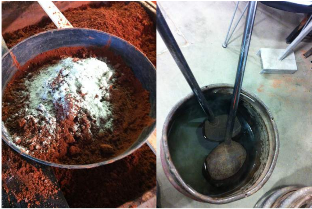
Figure 6. Example of mansfield sand with added bentonite, and ladles cooling down after use in the furnace, photography credit: JA Denton 2012
