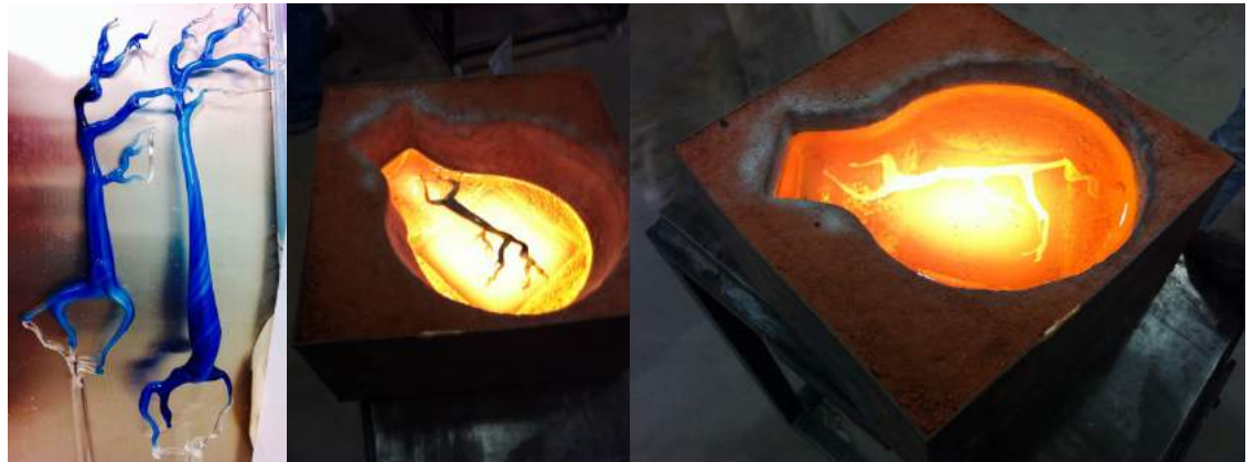
Figure 80. Floating inclusion process: left to right: Flameworked components, inclusion placed in cast between pours, inclusion sandwiched between glass substrate, 2012, photography credit: J A Denton
