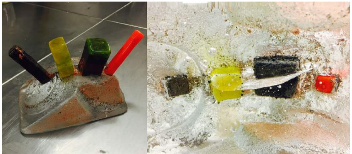
Figure 69 80mm test with solid System 96 transitional inclusion and Glasma furnace glass, 2015, photography credit: J A Denton
