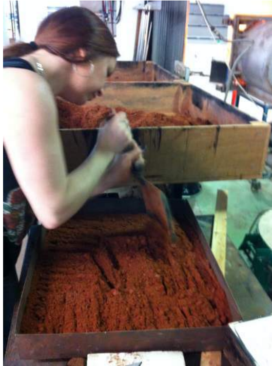
Figure 42 Preparing the Mansfield sand for casting, 2012. Photography credit: Anon
