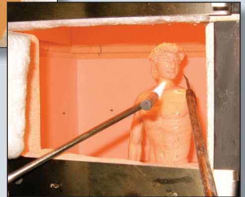
David assembly, process shot of parts of the statue assembled hot in a zone-controlled kiln.
